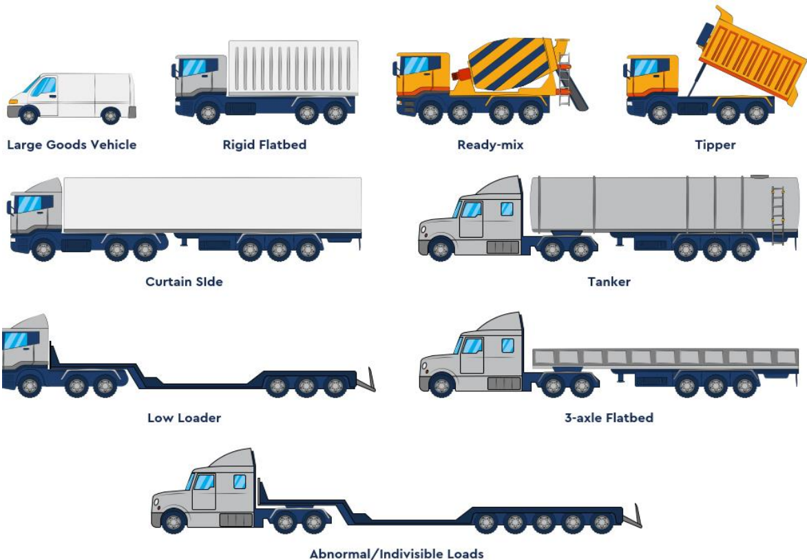
Figure 2-1 Construction Vehicle Types
